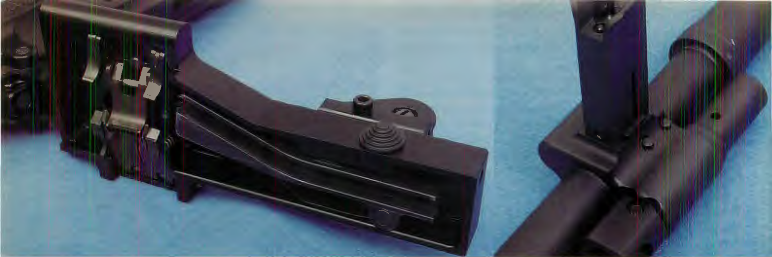
(left) Like most successful post-war light machine guns, the Shrike can trace its belt feed mechanism to the MG-42. (right) The Shrike's quick-change barrel also swaps out the gas system, so a fresh barrel is not mated with dirty operating components. The front sight is adjustable for both windage and elevation, allowing the barrel-zero to be pre-set by the operator. Adjustable gas regulator has four operating positions.
